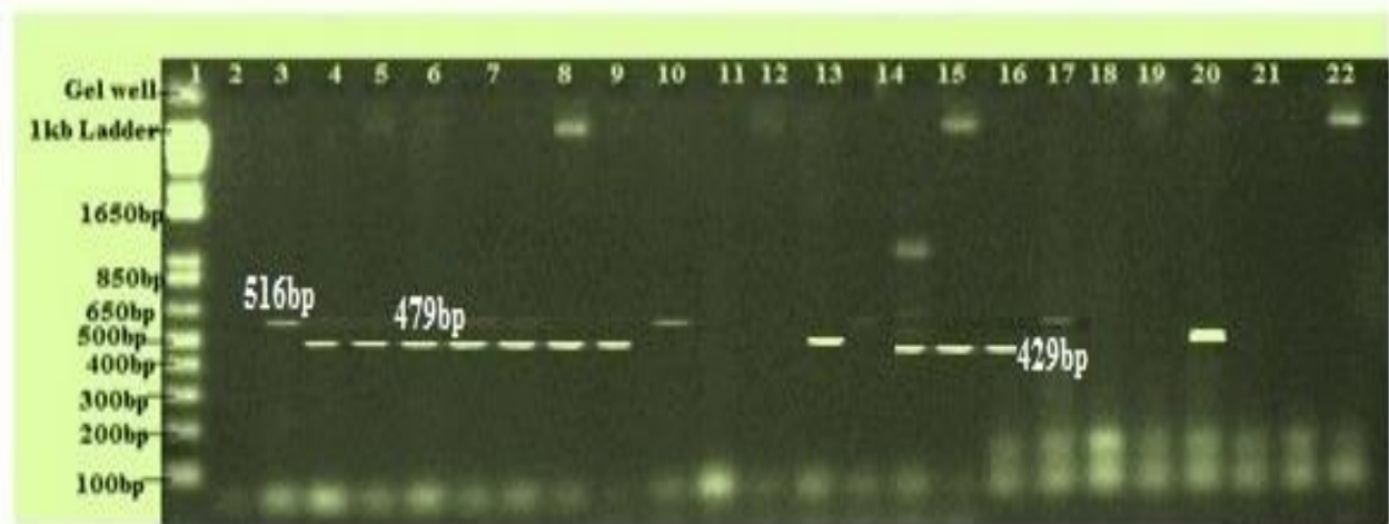
Plate II: Molecular characterization of the seven housekeeping genes { pta (479bp), gmk (429bp) and yqil (516bp)}.
