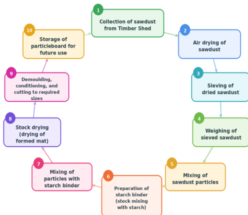
Figure 1: Process Cycle for sawdust Preparation and Particleboard Production
