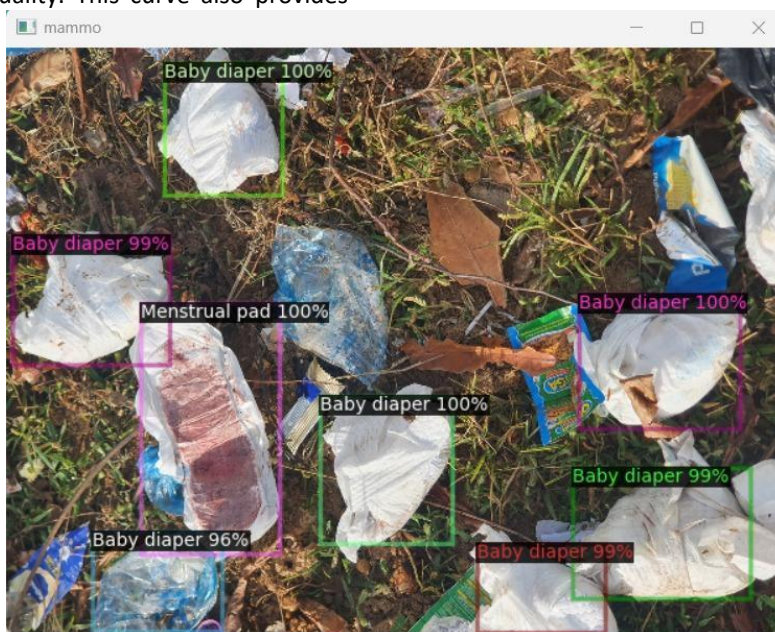
Figure 8: Sample detection output showing simultaneous identification of one menstrual pad and seven baby diapers with confidence scores from 96% to 100%
