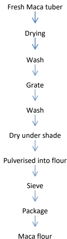
Figure 1: Process flow chart of maca flour Source: Sedano et al. (2017)
